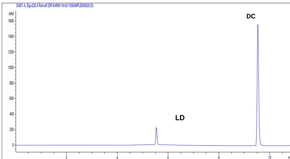
Fig. 3. HPLC chromatogram at 220 nm of a solution containing  $150 \mu\text{g mL}^{-1}$  DC and  $40 \mu\text{g mL}^{-1}$  LD obtained from Olfen® ampoules
