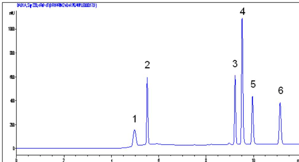
*Fig. 2.* HPLC chromatogram at 220 nm of a mixture containing: (1)  $50 \mu\text{g mL}^{-1}$  2,6-dimethylaniline (DMA); (2)  $100 \mu\text{g mL}^{-1}$  lidocaine hydrochloride (LD); (3)  $50 \mu\text{g mL}^{-1}$  2,6-dichloroaniline (DCA); (4)  $100 \mu\text{g mL}^{-1}$  diclofenac sodium (DC); (5)  $50 \mu\text{g mL}^{-1}$  N-chloroacetyl-N-phenyl-2,6-dichloroaniline (CPDCA); (6)  $50 \mu\text{g mL}^{-1}$  N-phenyl-2,6-dichloroaniline (PDCA)
