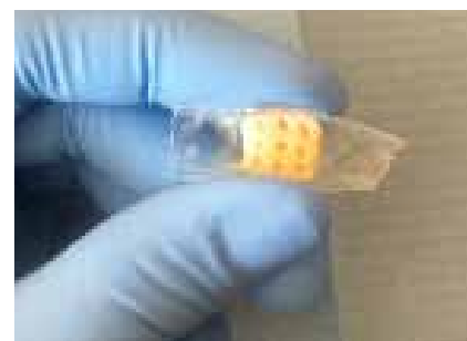
Fig. 3. Drill holes made into the resin of the stent.
