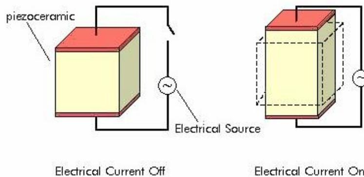
Figure1 showing voltage changing the shape of the solid (up to 4% in volume)
