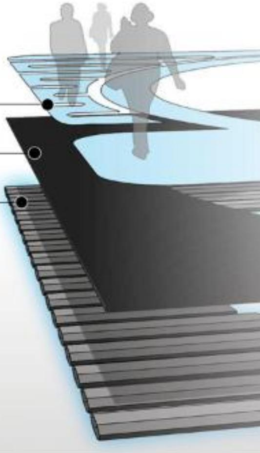
In Israel, a company called Innowattech is installing **strips of asphalt** embedded with piezoelectric materials. According to the company, the generators could produce 1 MWh of electricity from a four lane highway, or enough to power 2,500 homes.
