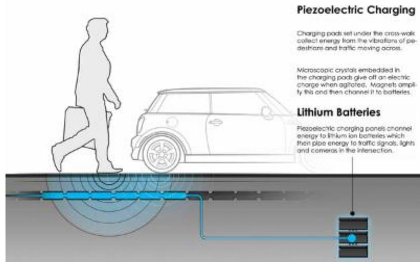
Figure3 Piezoelectric flooring.
