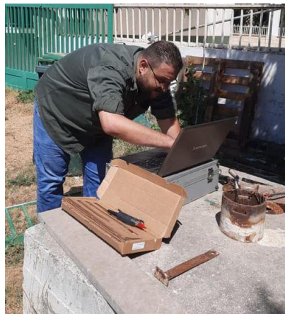
Setting the monitoring probes of ground water at el-Marj
